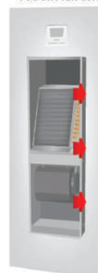
Step 6 Install Unilux retrofit fan coil
